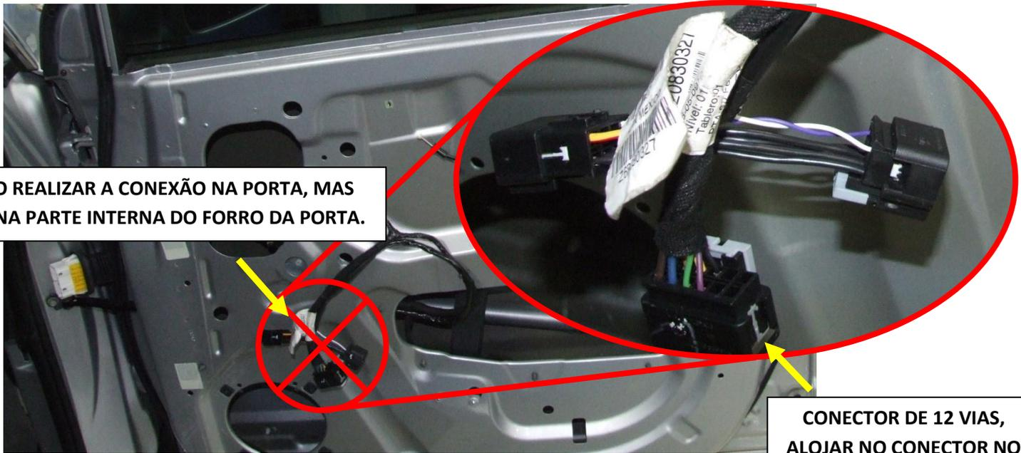
**NÃO REALIZAR A CONEXÃO NA PORTA, MAS SIM NA PARTE INTERNA DO FORRO DA PORTA.**
